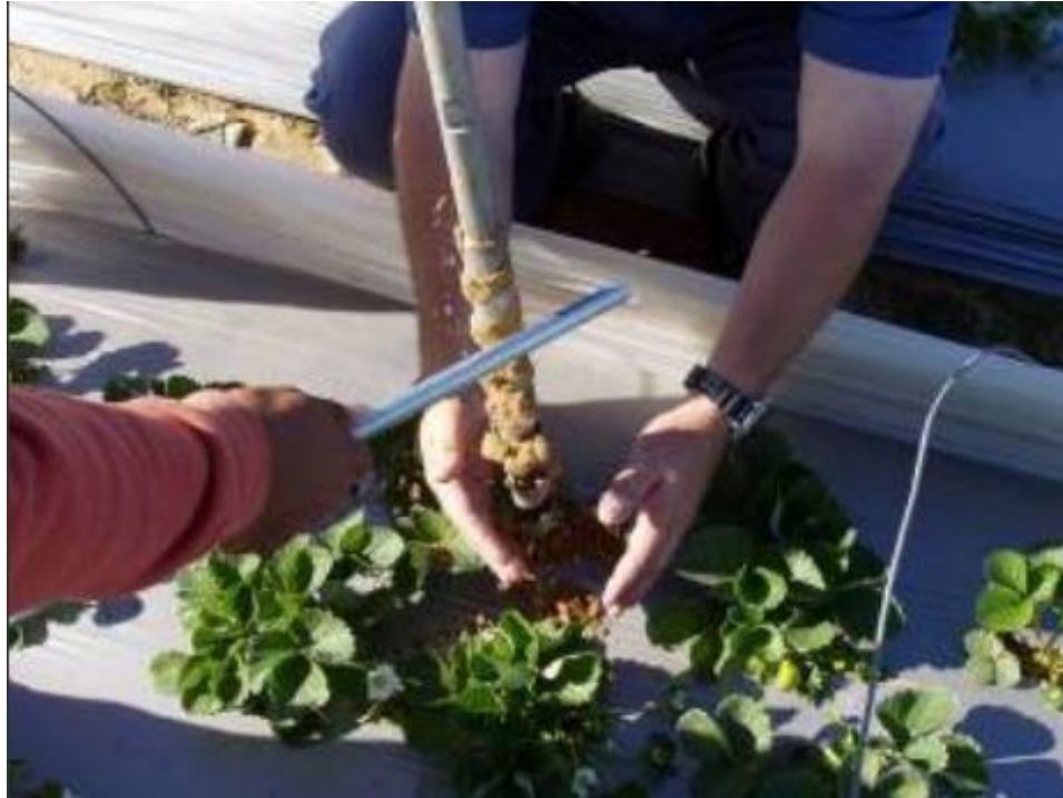
Figure 2: Collecting sand from the augured hole
