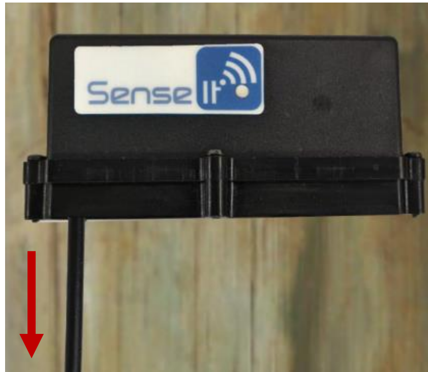
Figure 7: Logger installed with cable pointing down
